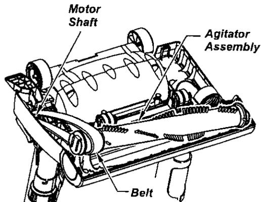
If the belt is still attached to the motor shaft, there will be tension on the agitator. If the belt is not broken, remove it from the motor shaft before lifting the agitator.
